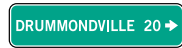
Code: I-100-1 Grandeur: 600 x 150 mm, 900 x 150 mm, 900 x 300 mm, 1200 x 300 mm, 1500 x 300 mm
