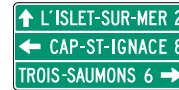
Code: I-100-3 Grandeur: 600 x 450 mm, 900 x 450 mm, 900 x 600 mm, 1200 x 600 mm, 1500 x 750 mm
